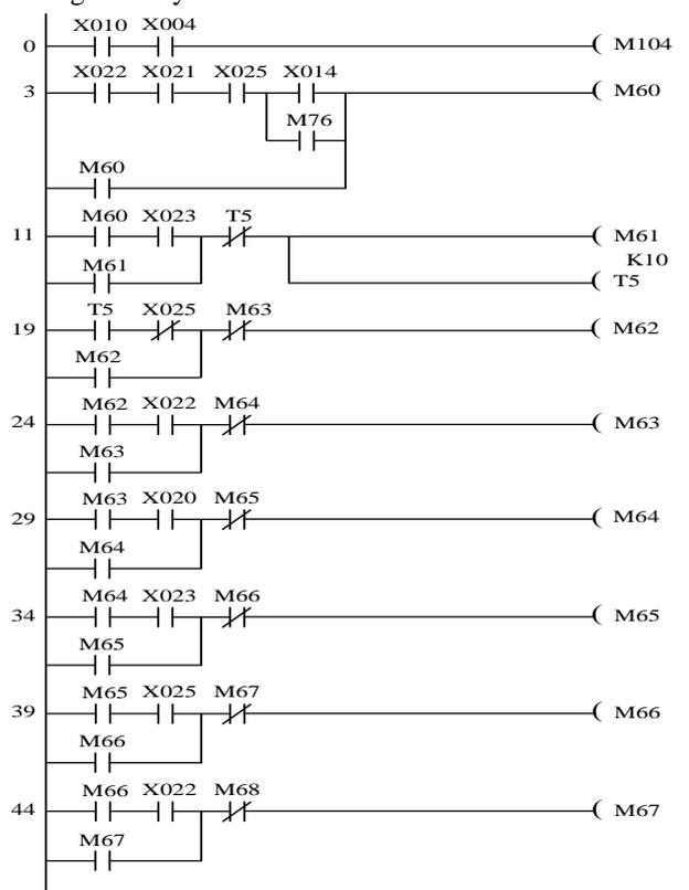
Fig.3. Partial ladder diagram for continuous operation mode
